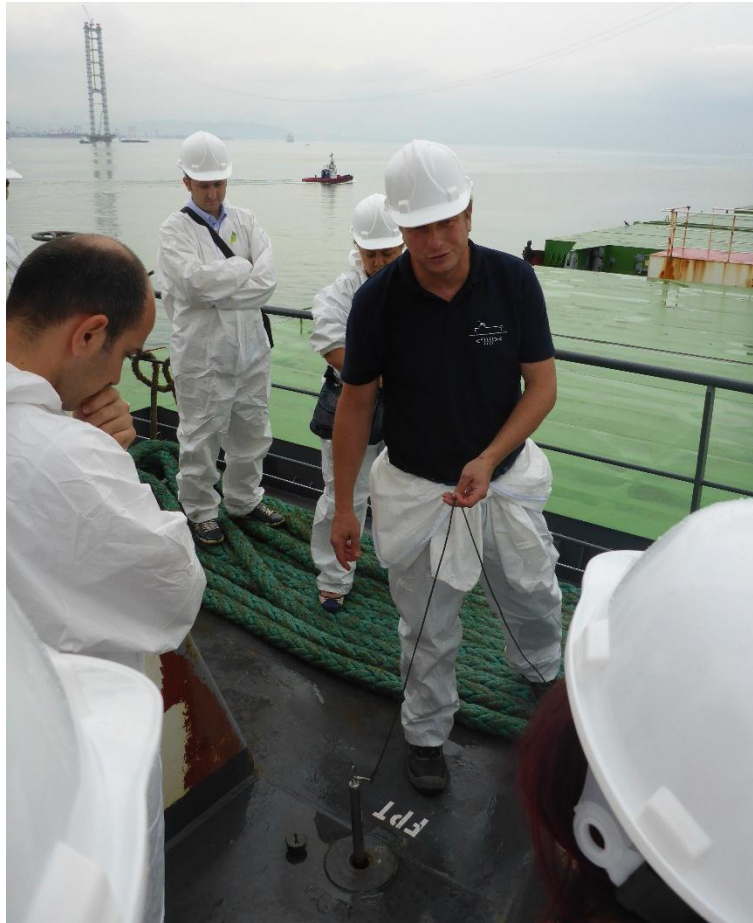
Picture 2 : Samples were taken from the tank through a sounding pipe using a water column sampler
