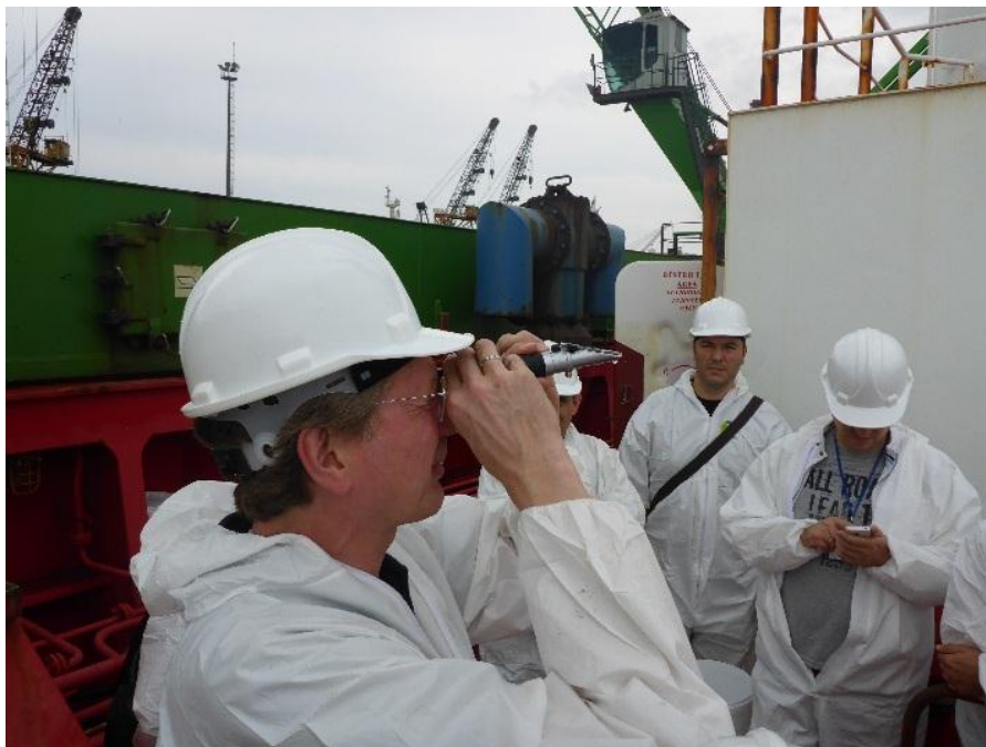
Picture 3 : Measuring salinity using a simple refractometer
